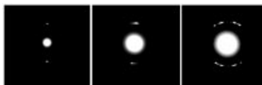
Fig. 3 SAED patterns of a mesoporous silica film grown at the boundary between air and water. Effective aperture diameters, left to right SAED patterns: 0.5 \mu\text{m} (spot), 1.5 \mu\text{m} (streaked), and 6 \mu\text{m} (arcs).
